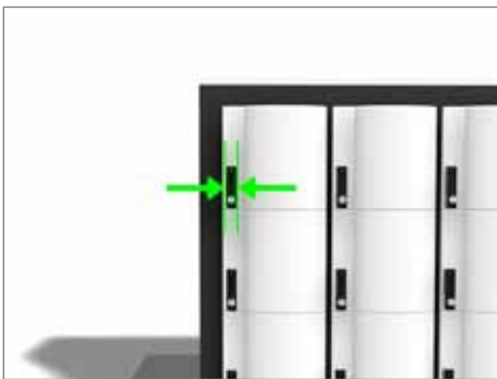
Example: Cabinet doors that curve outwards
